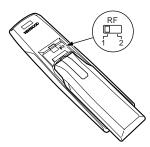
After changing remote control's RF frequency, you also must change the receiver's RF reception frequency.
